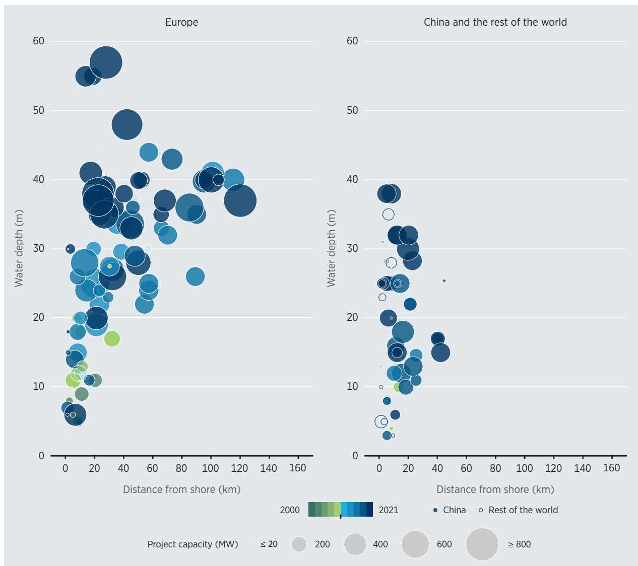
Figure 4.2 Average distance from shore and water depth for offshore wind in China, Europe and the rest of the world, 2000-2021
