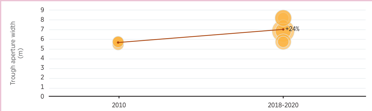
Figure B5.1 Trough aperture width trends for PTC CSP plants (2010-2018/2020)
