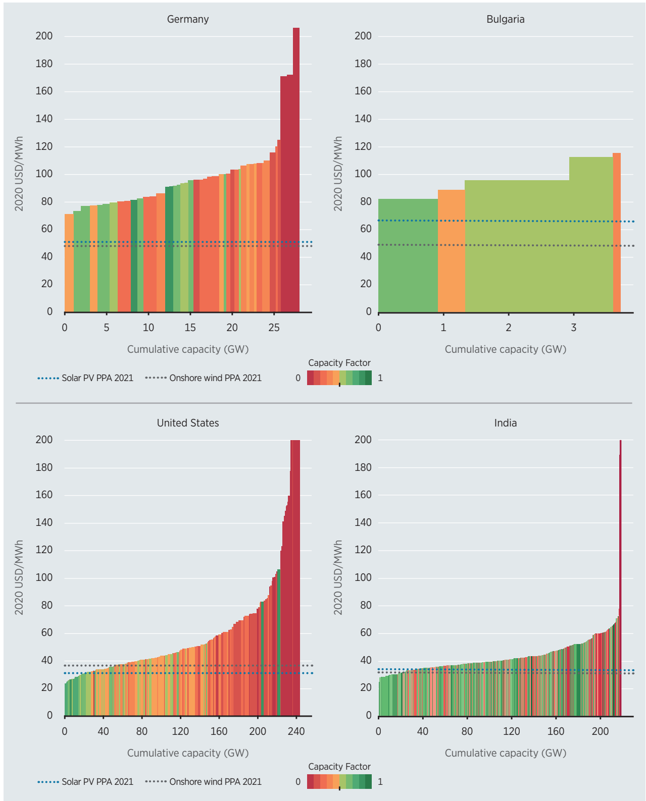
Figure 1.10 Operating costs only of existing coal-fired power plants in Bulgaria, Germany, India and the United States by installed capacity and capacity factor in 2020
