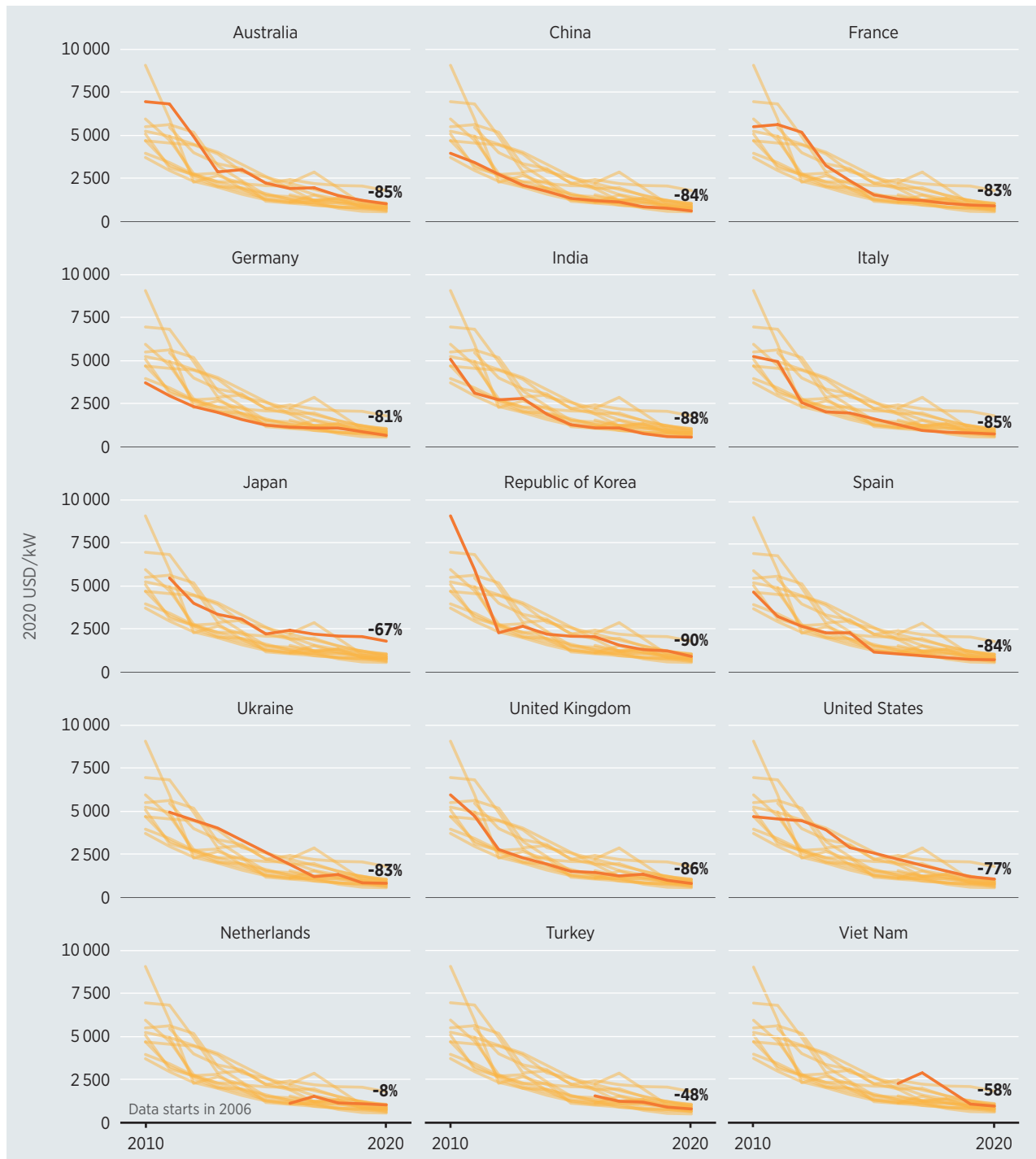
Figure 3.4 Utility-scale solar PV total installed cost trends in selected countries, 2010-2020
