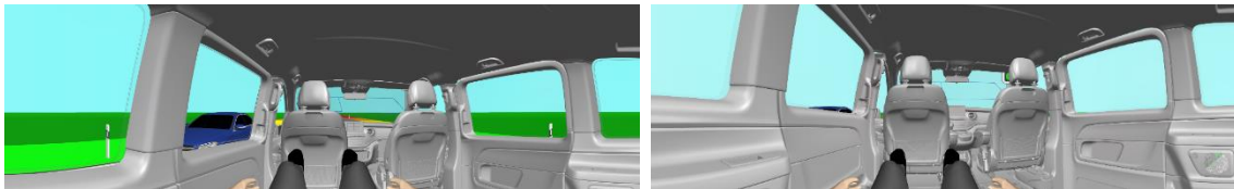
Fig. 7-11: Lying position with a lower H30 value: 95 th mannequin with 62° backrest angle – vision simulation. Modified from Daimler AG (2020)
