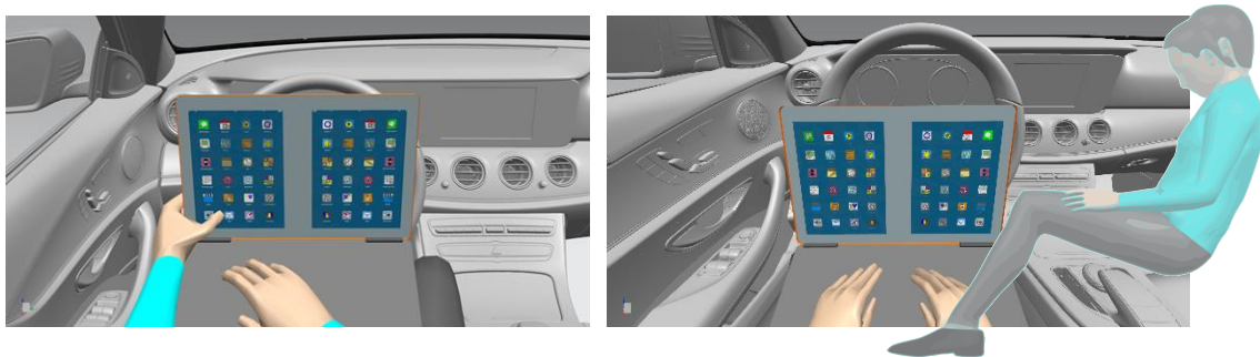
Fig. 5-3: Vision simulation representing NDRTs in upright sitting condition i.e. working on a laptop: 95 th male (left); 5 th female (middle); head-neck bending at cervical joint sitting upright (right) – first investigation. Modified from Daimler AG (2020)
