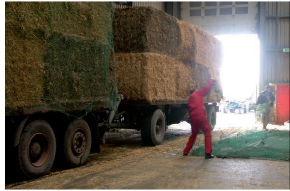
Figure 8.9. During unloading the driver and or employee at the heating plant remove the net. This gives an exposure to dust and spores from the straw [110]
