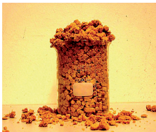
Figure 3.17. The swelling effect of water application to pellets.
