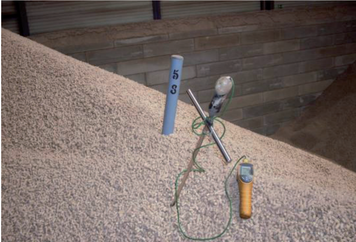
Figure 3.15. Temperature spears could be used for checking the temperature in the upper layer of bulk storage in e.g. a flat storage. The spears are often 2-3 m long and are introduced manually into the stack. The picture shows two different spears: one with a hand-held instrument and one (blue) transmitting the data wirelessly to a controller unit (Courtesy of Sensite Solutions B.V.)
