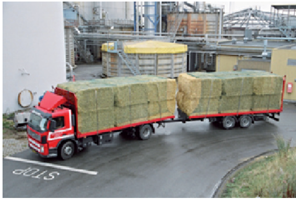
Figure 8.8. Truck with 24 big bales of straw waiting for unloading at a Danish straw pellet factory. The bales are arranged at the truck and at the trailer so the automatic crane in the straw storage can remove the bales from the truck in 2 lifts with 12 bales in each lift. (Photo: Lars Nikolaisen)
