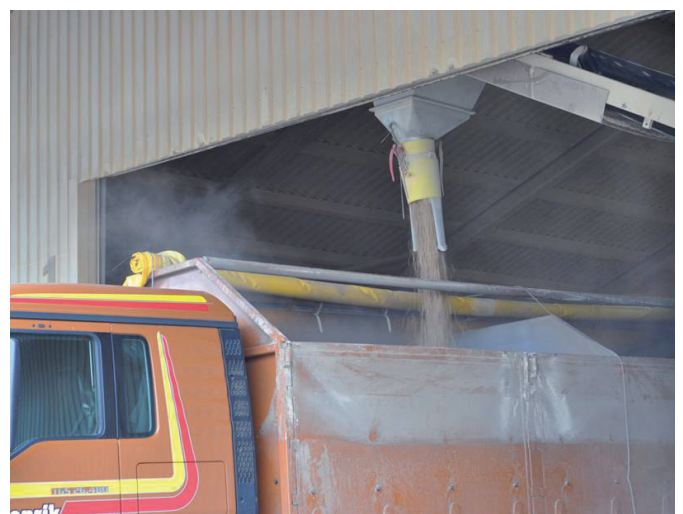
Figure 8.2. Loading of wood pellets in a truck at indoor storage with conveyor belt causes a high dust load in the vicinity [158].
