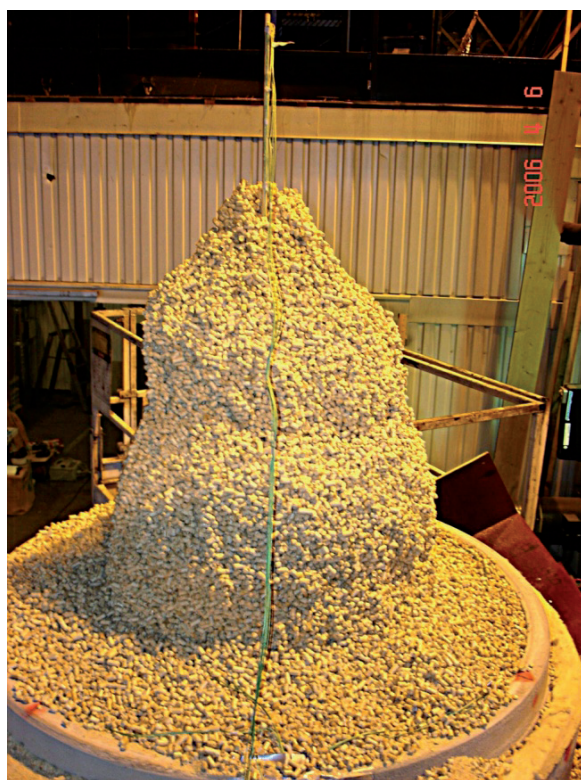
Figure 3.11. Agglomerated pellets about 1 m above the pyrolysis zone in the test silo [146].
