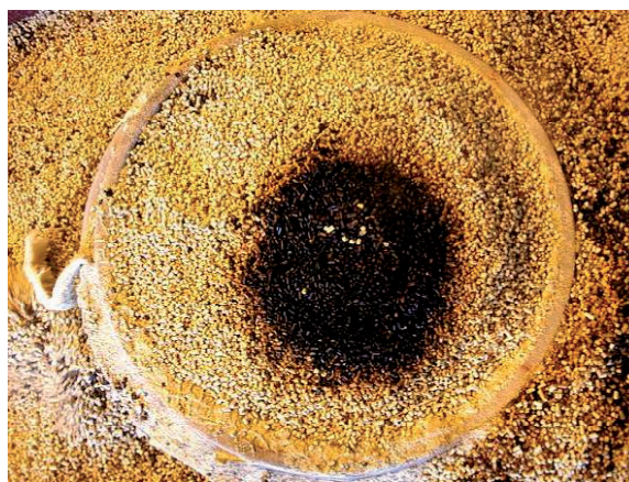
Figure 3.12. Pyrolysis zone about 0.5 m below the ignition source in the test silo [146].
