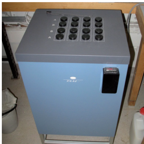
Figure 3.4. Left: The eight channel TAM Air 3116-2 isothermal calorimeter. Right: Examples of pellets samples in glass ampoules.
