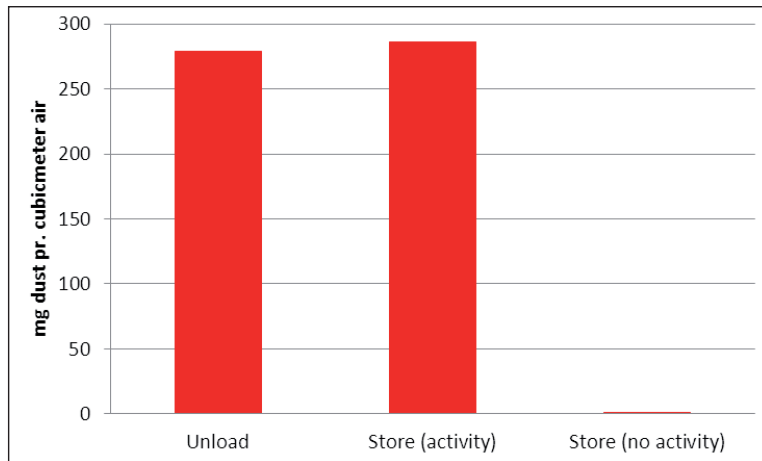
Figure 8.3. Wood dust load (mg / m 3 air) by unloading pellets (left bar), see Figure 8.4. The dust concentration is many times the limit values as indicated in Table 8.1. The middle bar shows the dust load in a storage with different transport activities with pellets. The dust concentration is again many times the limit value. The right bar shows the dust load in a storage without activities [158].
