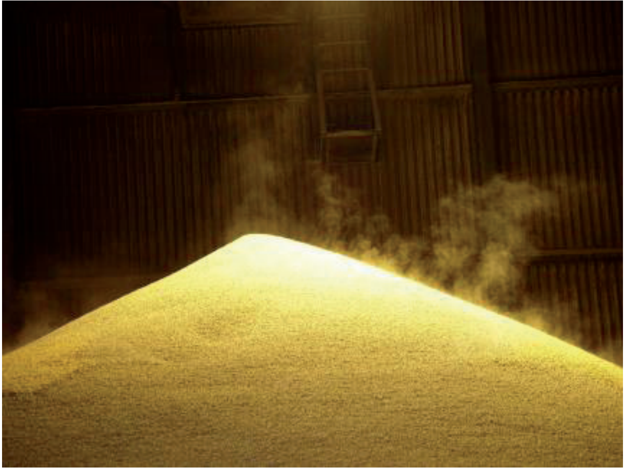
Figure 3.1. A stack of freshly produced pellets in a flat storage where the pellets have elevated temperatures due to self-heating of the pellets. The "smoke" visible on the picture is probably a combination of water moisture and various gases (off-gassing); (courtesy of Ingvar Hansson, Swedish Civil Contingencies Agency)
