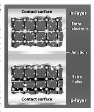
an abundance of electrons, which have a negative electrical charge. The other layer is a "p-type" semiconductor with an abundance of "holes," which have a positive electrical charge.
